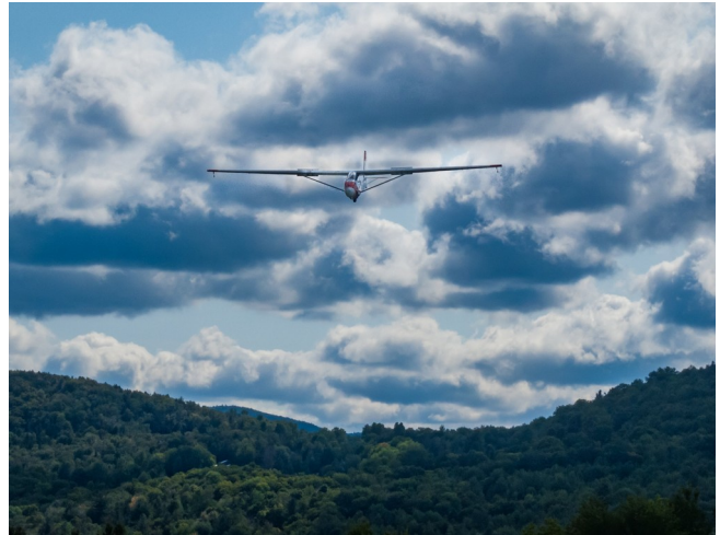
Schweizer 2-23 on landing approach with spoilers deployed
