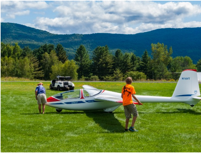
A PW-6U sailplane balancing on one wheel while being lined up
