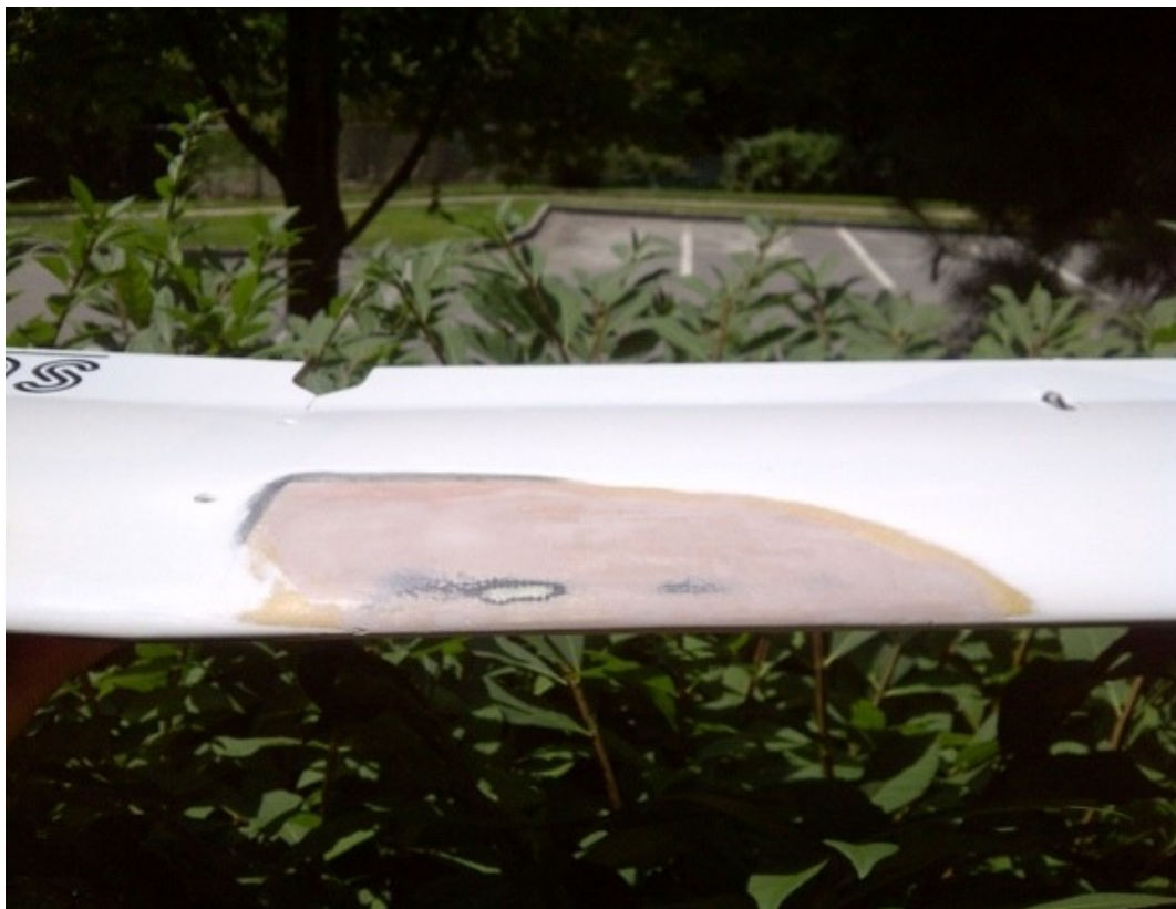
Sanded between applications of thin layers of Bondo. Yup, the carbon fiber layer was a tad high in one spot of the D-channel, but not anymore. It's okay; it has fiberglass underneath. The black edge in the rear of the repair is where the paint was feathered down to the carbon cap on the spar.
