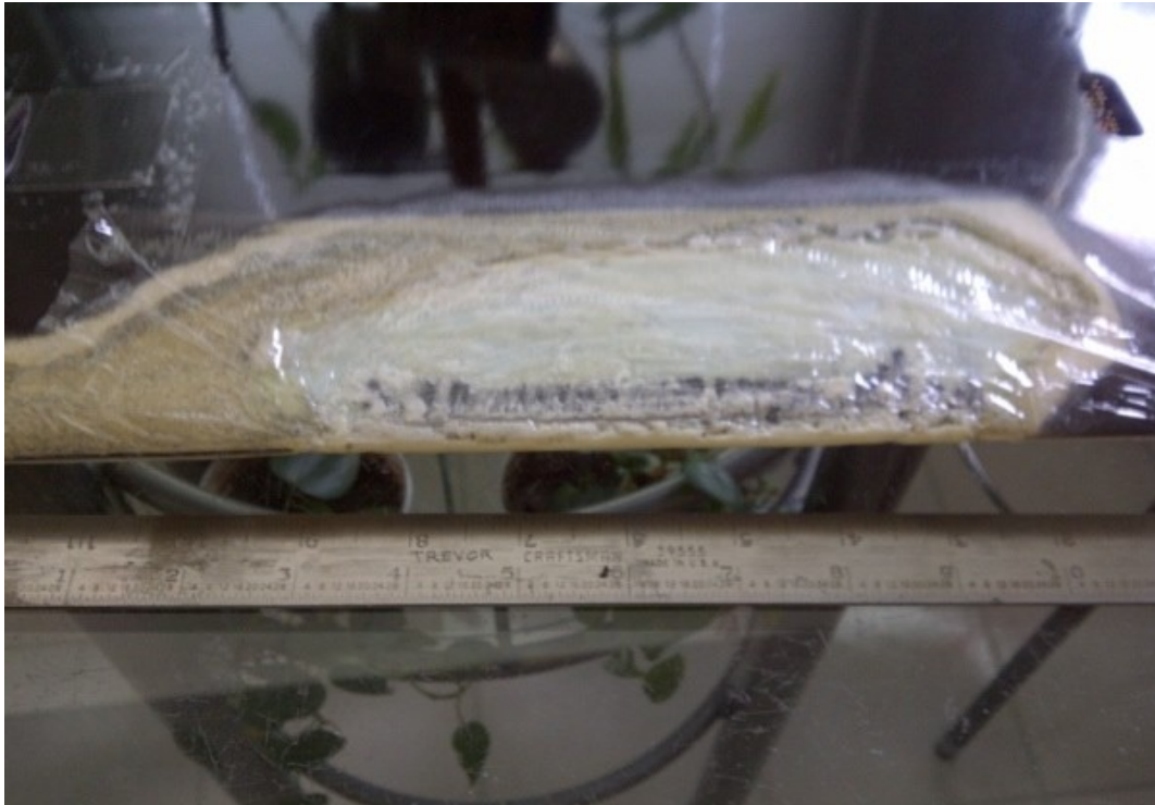
Saran Wrap and rolling a steel ruler over the leading edge forms the foaming glue into a shaped leading edge and really cuts back on sanding after it hardens.
