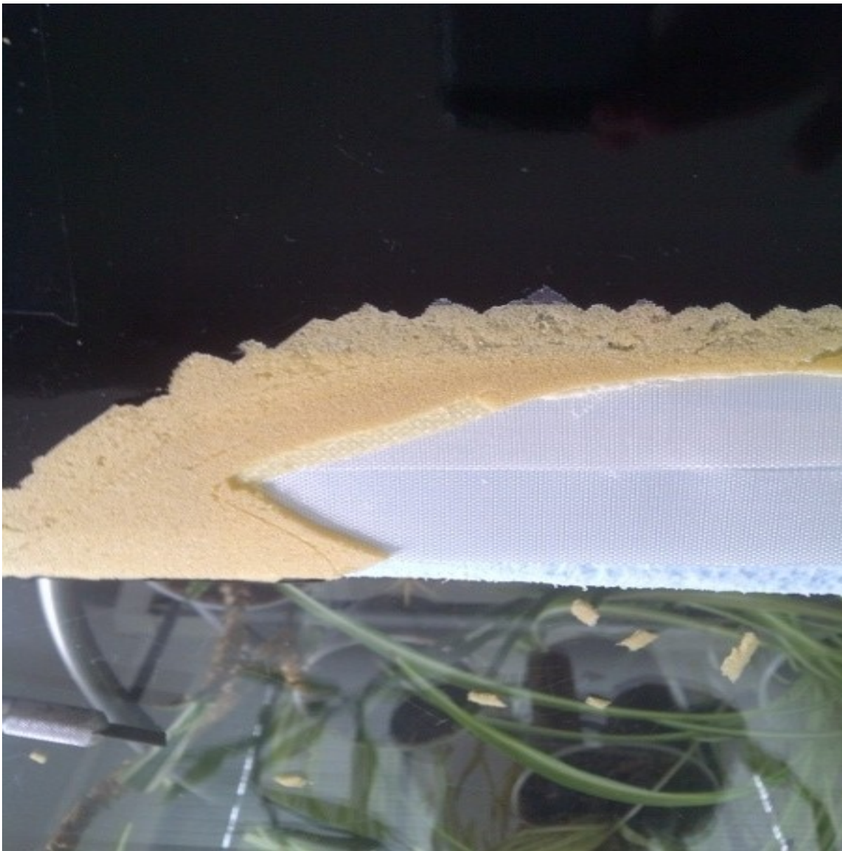
Fiberglass is inserted between the blue foam plugs and the inside of the wing. The outside layer of the wing's yellow foam is being cut away at the edges so that the fiberglass can be epoxied to the Kevlar netting at the same time the fiberglass is laminated to the blue foam plugs.
