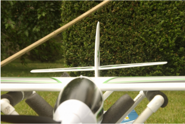
The stabilizer was not parallel with the wings
